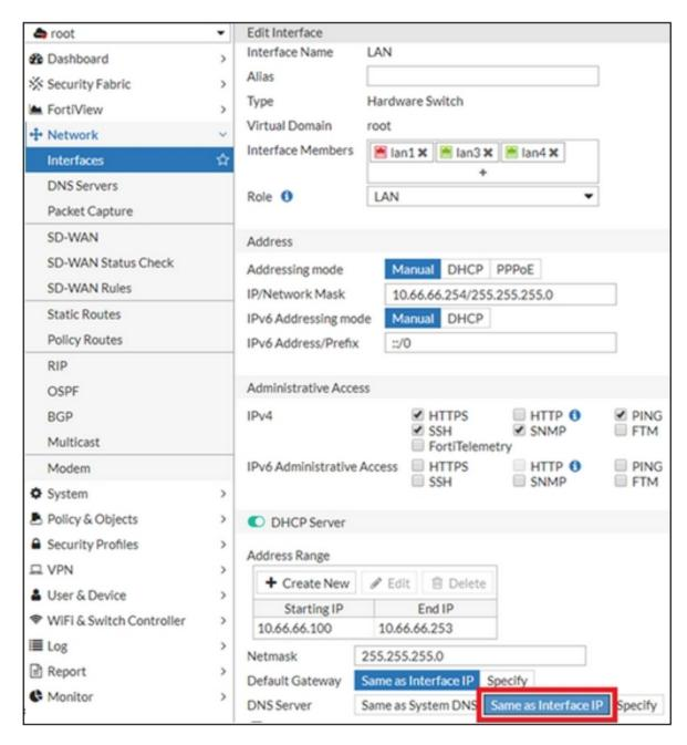
Technical Note: DNS resolution not working when DNS Server configured to 'Same as Interface IP'
