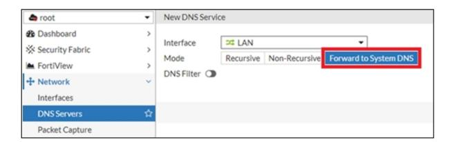
Technical Note: DNS resolution not working when DNS Server configured to 'Same as Interface IP'
