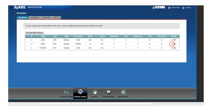
Change the two options highlighted below, change the mode to Bridge and select enable VLAN and then set 802.1q to be 101. Once done hit ok to save the config
