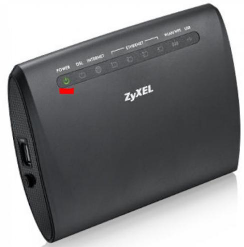
Once the above step is completed and the power light is solid, then you can take the yellow RJ45 cable inside the routers box (you can use your own if this one is not long enough) and connect one end to any LAN port on the back of the router. The other end is connected to your network device such as your PC/Laptop.
