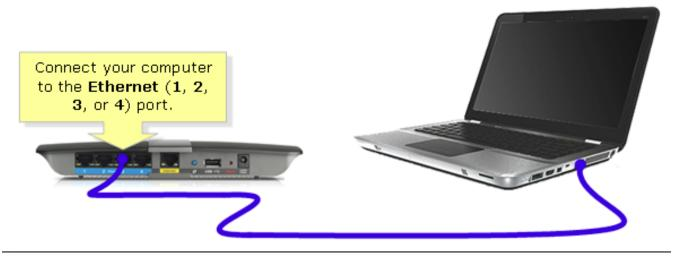
Yes the router in the picture is different to yours but the concept stays the same. The port numbered 4 cannot be used for a connection to a network device as it will be used to connect your modem to the router and covert the telephone line data into Ethernet.
