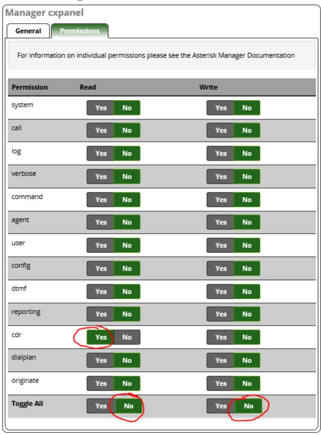
NOTE: ONLY select the permissions you need to and be very careful with write, remember to air on the side of caution to keep your system as secure as possible at all times and also LOCK IT DOWN to only the IP addresses you need.
