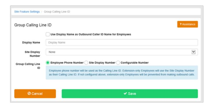
To set a default Site Display Number for HSIPT Trunking Users needed to allow and HSIPT Trunking Users to make external calls:
